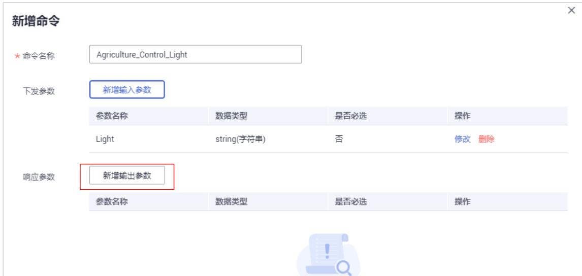
The screenshot shows the 'Add Command' dialog box. In the '下发参数' (Downstream Parameters) section, there is a table with one row: Light (string type, optional). In the '响应参数' (Response Parameters) section, there is a button labeled '新增输出参数' (Add Output Parameter) which is highlighted with a red box. Below this button is another table where the first column is '参数名称' (Parameter Name) and the second column is '数据类型' (Data Type).
