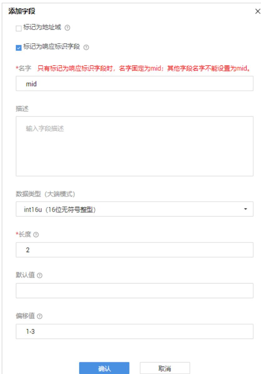
The screenshot shows the 'Add Field' dialog. Under 'Field Properties', the 'Mark as Response Identifier Field' checkbox is checked. The field name is 'mid'. In the 'Description' section, there is a placeholder 'Input field description'. Under 'Data Type (Big-endian mode)', the type is 'int16u (16-bit unsigned integer)'. The 'Length' is set to '2'. There are empty fields for 'Default Value' and 'Offset'. At the bottom are 'Confirm' and 'Cancel' buttons.
