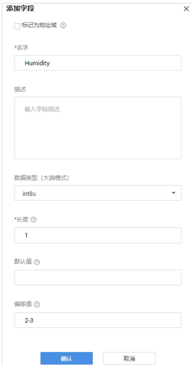
The screenshot shows the 'Add Field' dialog box with the field name set to 'Humidity'. Other settings include: Description: '输入字段描述', Data Type: 'int8u' (Big-endian mode), Length: '1', Default Value: empty, and Offset: '2-3'. At the bottom are 'Confirm' and 'Cancel' buttons.
