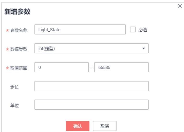
The screenshot shows the 'Add Parameter' dialog box. It has fields for '参数名称' (Parameter Name) set to 'Light\_State', '数据类型' (Data Type) set to 'int(整型)', '取值范围' (Value Range) set to '0 - 65535', and '步长' (Step) and '单位' (Unit) both empty. At the bottom are '确认' (Confirm) and '取消' (Cancel) buttons.
