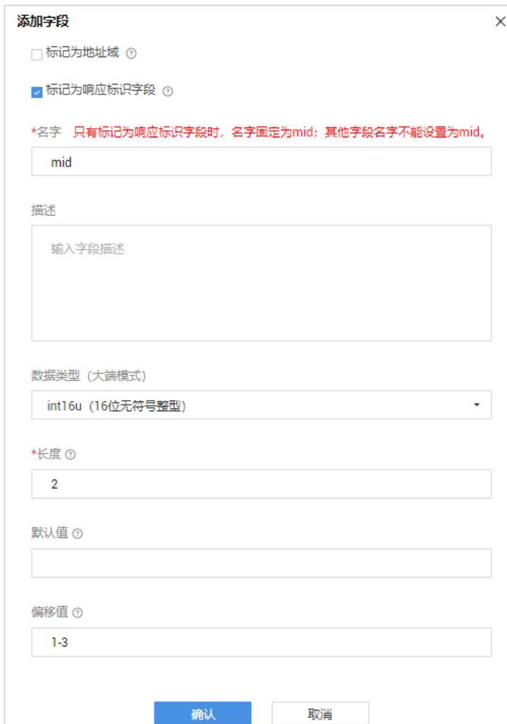
The screenshot shows the 'Add Field' dialog box with the 'Mark as Response Identifier Field' checkbox checked. The field name is 'mid', and the data type is 'int16u (16-bit unsigned integer)'. Other fields like length (2), default value, and offset (1-3) are also filled. The 'Confirm' and 'Cancel' buttons are at the bottom.
