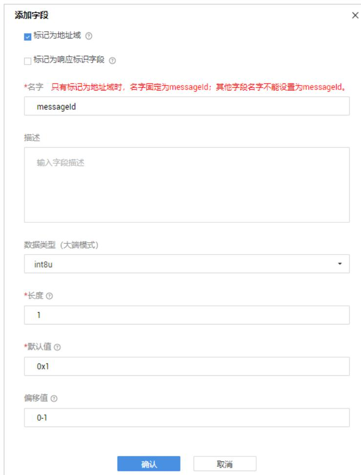
The screenshot shows the 'Add Field' dialog. The 'Address Domain' checkbox is checked. The 'Name' field contains 'messageId'. The 'Description' field is empty. Under 'Data Type (Big-endian mode)', 'int8u' is selected. The 'Length' field contains '1'. The 'Default Value' field contains '0x1'. The 'Offset' field contains '0-1'. At the bottom, the 'Confirm' button is highlighted by a blue box.
