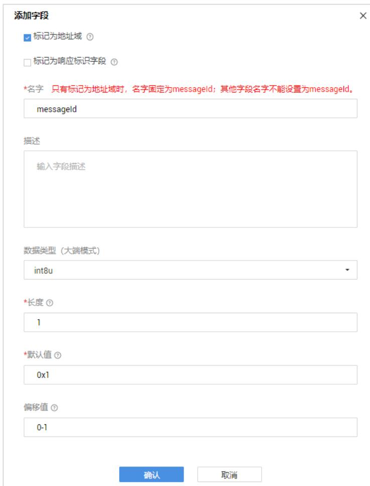
The screenshot shows the 'Add Field' dialog. Under the 'Address Domain' section, the 'Check' box is checked. The field name is set to 'messageId'. In the 'Description' section, the placeholder text is 'Input field description'. Under 'Data Type (Big-endian mode)', the selection is 'int8u'. The 'Length' is set to '1'. The 'Default Value' is '0x1'. The 'Offset' is '0-1'. At the bottom, there are 'Confirm' and 'Cancel' buttons.
