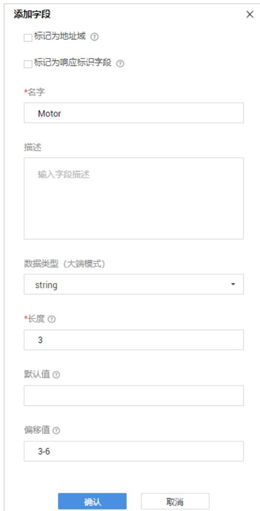
The screenshot shows the 'Add Field' dialog. It includes fields for marking it as an address domain or a response identifier, a name input field containing 'Motor', a description input field, a data type dropdown set to 'string', a length input field set to '3', a default value input field, and a offset input field set to '3-6'. At the bottom, there are 'Confirm' and 'Cancel' buttons.
