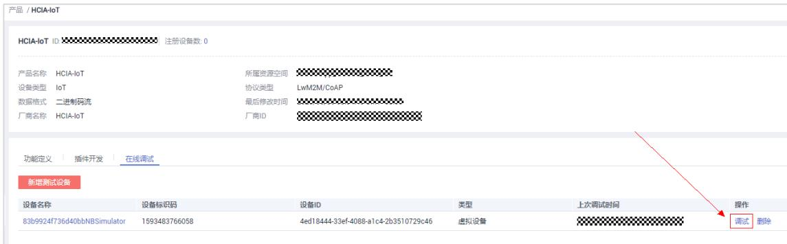
The screenshot shows the HCIA-IoT device management interface again. It displays the same device details as before. Below the tabs, the table now includes a column for 'Last Debug Time' (上次调试时间) and an 'Operations' (操作) column. A red arrow points from the text 'Click the "Debug" button on the right side of the device' (点击设备右侧的“调试”按钮) to the 'Debug' (调试) button in the 'Operations' column for the first device listed in the table.
